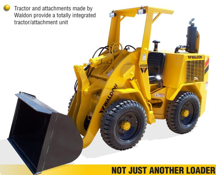
The ultra-compact, heavy-duty, articulating, 4-wheel drive Waldon 4500B Unitractor has an SAE operating capacity of 1400 lbs. This unit was designed for low clearance heavy industry, mining, material handling applications with abusive environments. This loader is designed and manufactured in the U.S. by the original compact articulating loader manufacturer.
