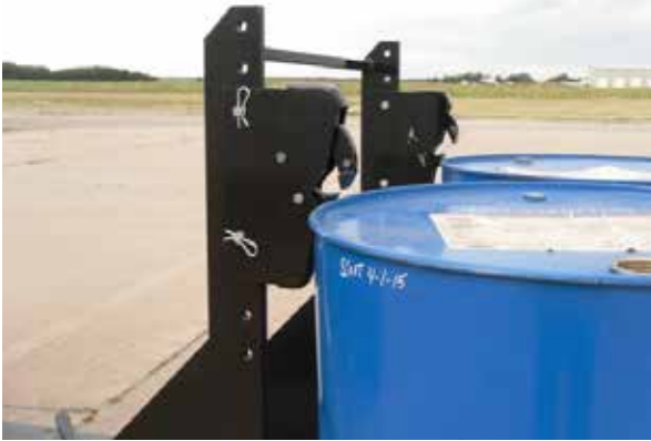
Drive up to the drum and lower the heads over top ring on the drum
