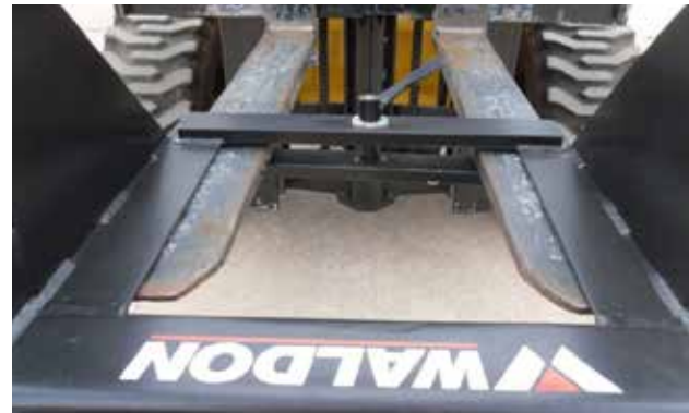
Drum handler attaches to the forks with 3/4" thick bar
