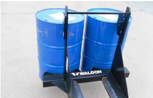
Drive up to the drum and lower the heads over top ring on the drum
