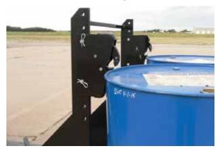
Drive up to the drum and lower the heads over top ring on the drum
