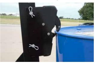
Head automatically grips the ring of the drum as you lift up the handler
